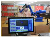
All movements are displayed on the interactive GUI, which sends out warnings when the pallets need restocking or the waste bin is full.
