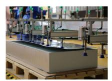
Printing plates are stacked emulsion side down on a pallet. Sensors detect the height and position of the stack. The front of the picking arm lifts up the plate.
