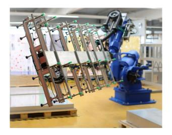
Saving time and space, the Robotic Plate Loader automates multiple manual, repetitive tasks, such as loading plate cassettes used in autoloaders or fixing pallets on the base frame of skid loaders. In fact, this robot replaces up to two autoloaders and two skid loaders, improving working conditions for operators as well as reducing the overall equipment footprint by at least 20 to 30%.
