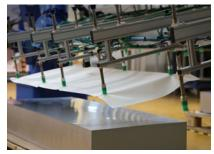
The picking arm turns  $180^{\circ}$  to pick up the interleaf with the other side.
